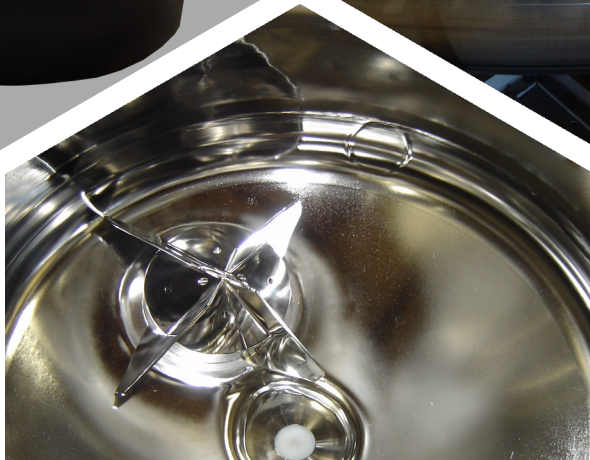
Inside of small mixing vessel showing final electro-polished surface after mechanical and chemical finishing processes.
