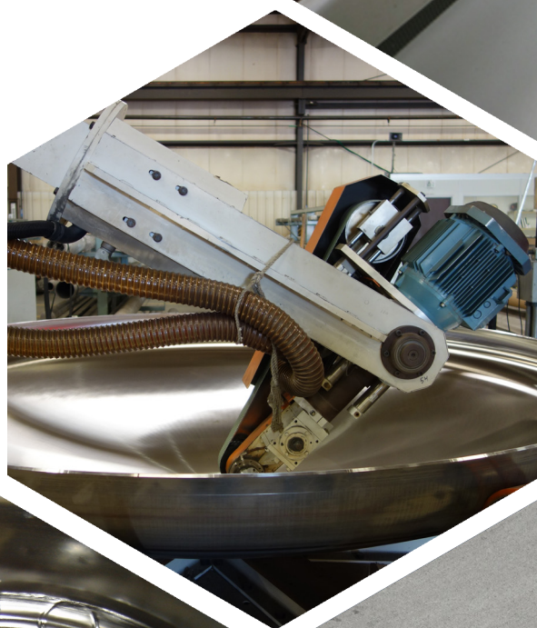
Robotic polishers use an abrasive material (measured by grit coarseness) to create the finish.
