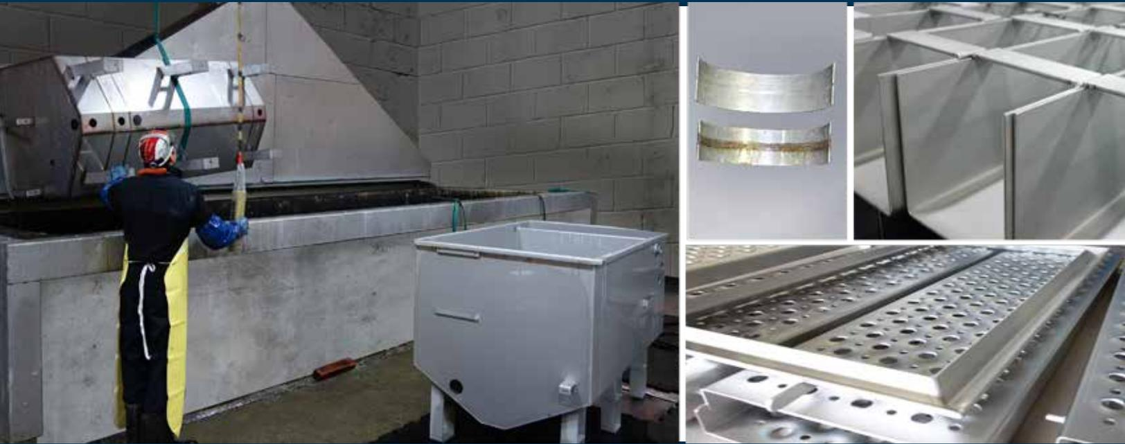
**Pickle Passivation** is the immersion of metal in a pickling bath or coating with nitric-hydrofluoric acid. Pickle passivated stainless material has a light matte appearance. Customers use Apache's in house passivation services for:
